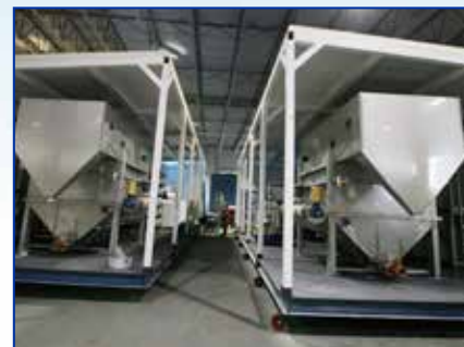
4-part package plant for sewage treatment for 7500 person work camp
