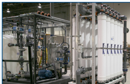
UF/NF system removes heavy metals from dredged seawater for release to environment
