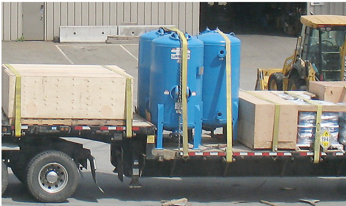
Greensand filtration vessels prepared for shipping to the Yukon, and during installation, top.
