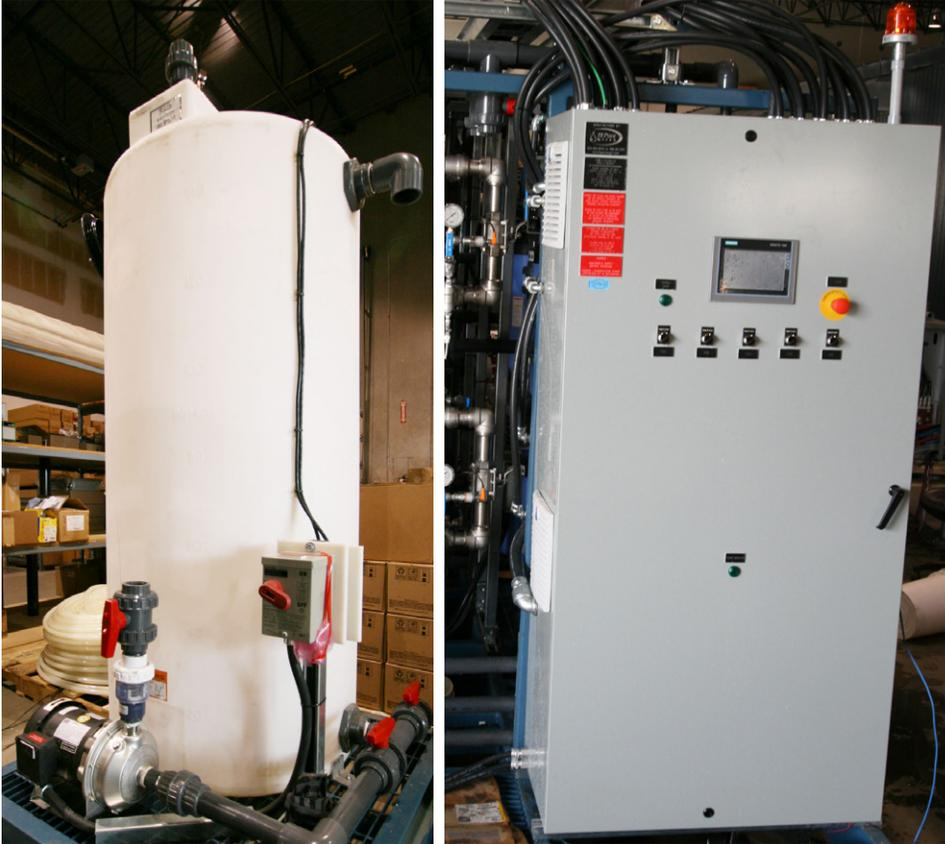
*Clean in Place system left and control panel with touchscreen HMI.*
