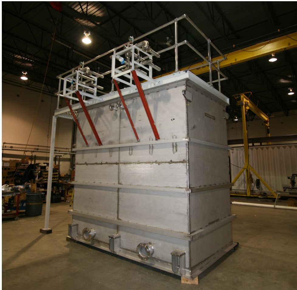
Fig. 1 - Stainless steel tank fabricated for Bend, Oregon MBR system.
