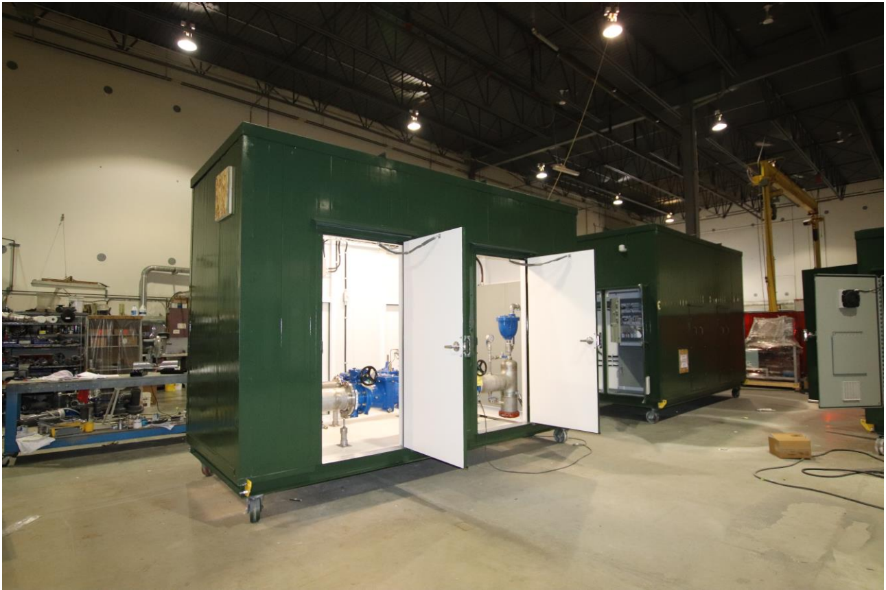
Figure 1 – Upper Bay View Road PRV Station with Installed Piping Assembly
