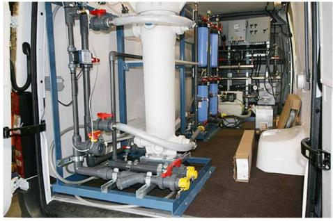
A bag filter, cartridge filters, activated carbon filters, ultraviolet units and chemical metering systems can be combined in the mobile water treatment pilot plant
