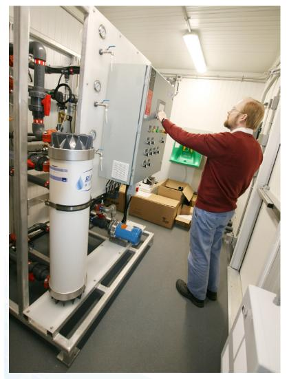
A higher capacity UF package plant, with chlorine and air injection systems for the membrane backwash, is prepped for shipping
