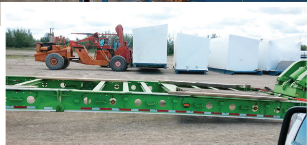
The water treatment plant arrives in four sections at Hay River, Alberta at the start of its Mackenzie River journey. Top: the re-assembled complete treatment plant in Cambridge Bay
