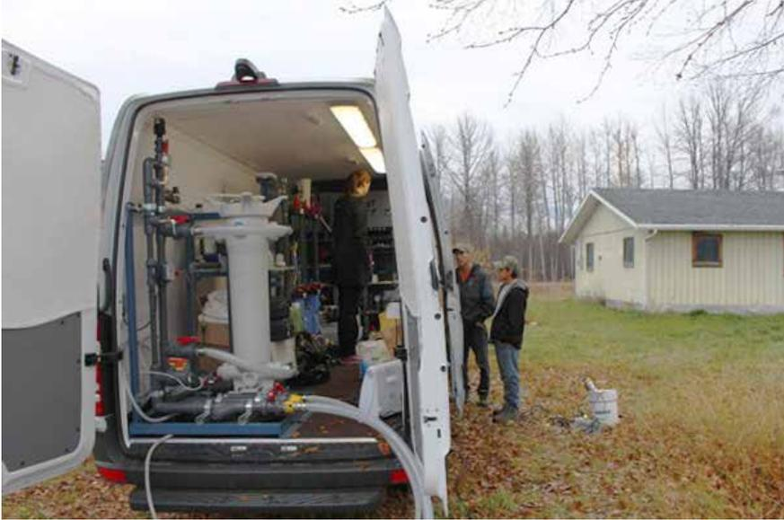
*Megan testing source water with the pilot plant at Middle River, BC*
