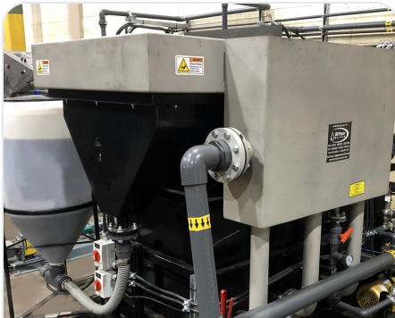
The DAF package, where oil, grease, and suspended solids get skimmed off the top.
