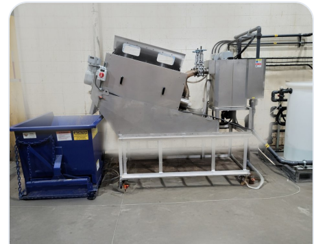
Dual screw presses turn DAF sludge into a cake dry enough to dump and haul.
